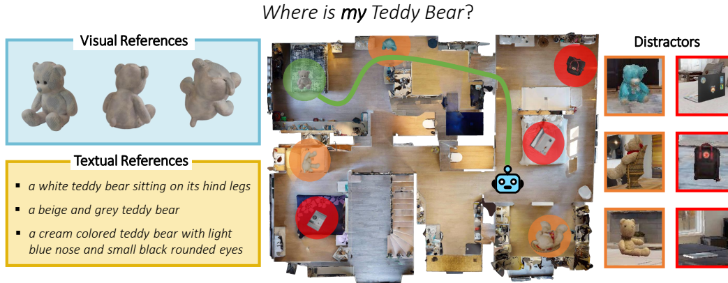
Figure 1: We introduce the task of Personalized Instance-based Navigation (PIN), where the agent is asked to navigate toward a personalized object instance using multimodal references and distinguish it from distractors ( i.e. , other objects of the same category as the target or of other categories). The target object, same category distractors, and other distractors are circled, respectively, in green, orange, and red. The total number of available objects in the dataset is 338, corresponding to different instances of 18 object categories.
